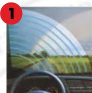
**1 Lace Curtains:** Arm defects or long periods in the 'park' position can deform the wiper blade edge, causing a veil effect across the windscreen.
