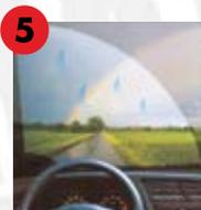
**5 Wind lift:** When travelling at high speed, the wiper misses parts of the windscreen, then the wiper blade or wiper arm should be replaced.
