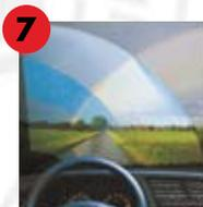
**7 Unwashed margins:** Deterioration of the wiper blade linkage, or decreased wiper pressure can result in parts of the windscreen not being wiped at all.
