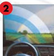
**2 Bands:** Wiper blade rubber can wear out or become damaged with age. This will result in thick bands of water being left on the windscreen.
