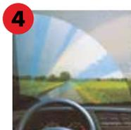
**4 Chatter hopping:** This happens when wiper blades judder across the screen leaving radial streaks. Chatter hopping can be caused by a deformed wiper element, worn blade linkage or a change in wiper arm characteristics.
