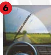
**6 Vibration judder:** A deformed wiper element, the wrong adaptor or wear and age on the wiper blade rubber and links can cause jerky wiper arm movement.
