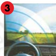
**3 Lines:** When the wiper rubber becomes damaged with age, or wears thin, fine semi-circular lines are left on the windscreen.
