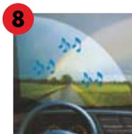
**8 Noise:** Noisy wipers may be a sign that the wiper element is deformed, or has hardened. This could also be caused by a worn wiper blade structure.
