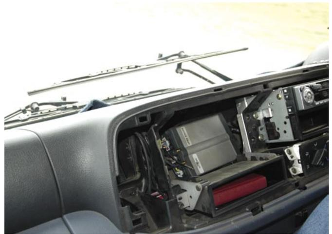
**Above:** The technician locates the tracking unit in the dashboard and disconnects the GSM.
